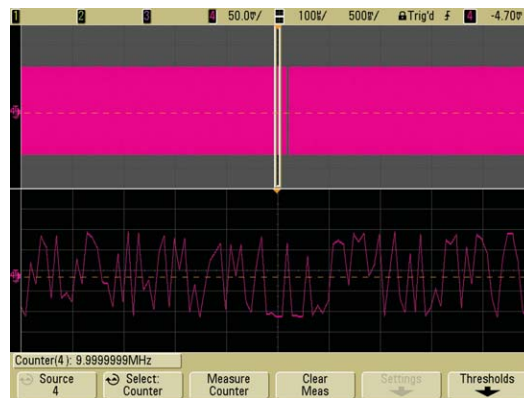
Figure 13. Built-in hardware counter allows for making 8-digit frequency measurement using an external 10 MHz reference input.
